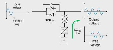
When the grid voltage returns to normal value, AVC-RTS stops working and controls the thyristor to turn on, the output voltage returns to the grid voltage, and the super capacitor begins to charge in preparation for the next voltage sag.
