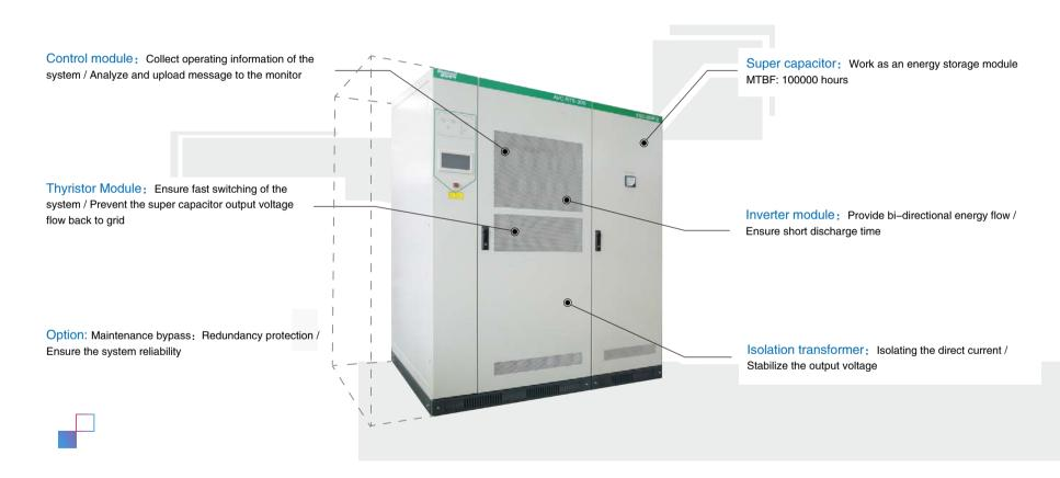
Perfect compensation 0~130% residual voltage to 100% rated voltage Fast switching time less than 100us, full response time less than 5ms Strong over-voltage regulation ability, rated voltage can be set between -15% and 15% Redundancy design with high reliability, free maintenance and low cooling cost of super capacitor
