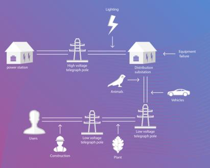
Voltage sag is generally caused by the failure of power grid, substation facilities or sudden large changes in load. In the process of long–distance transmission, there are many unpredictable situations, such as power system fault, lightning strike, large motor starts, capacitor switching and other events in the transmission and distribu–tion system.
